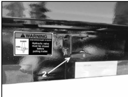
Deck Control Valve
