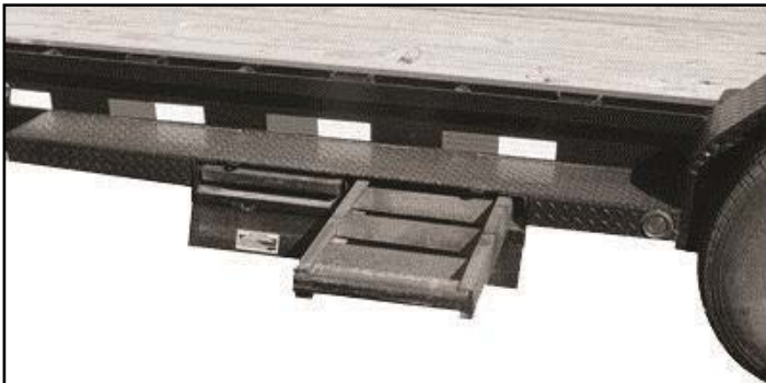
Side Storage Position Ramps
